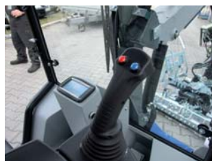
Easy to understand control elements with optimum view of the clamp/paving edge
